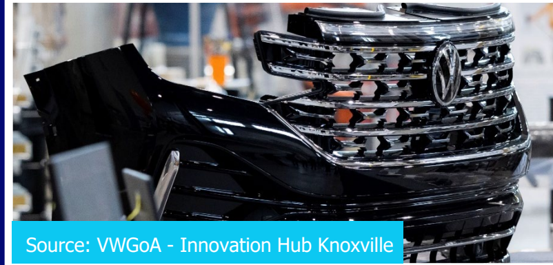
Fully assembled VW ATLAS bumper with 60% PureFive™ resin Status: Proof of Concept – Not Yet Commercialized
